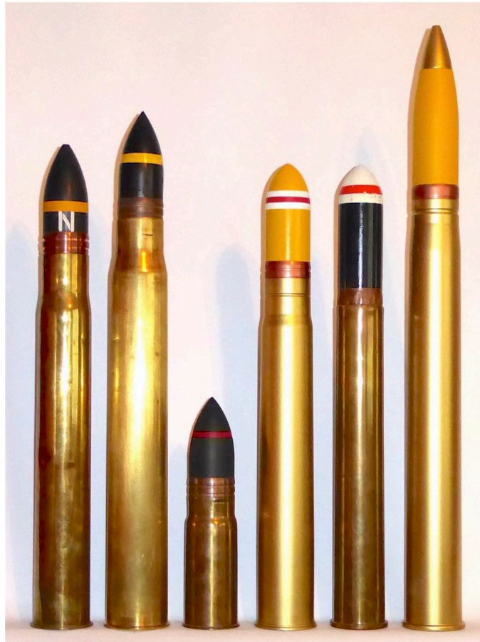
Photo: 47x376R 3^{\text{PR}} Hotchkiss; 47x413R 3^{\text{PR}} Vickers; 47x131R 2\frac{1}{2}^{\text{PR}} Hotchkiss; 47x351R 3^{\text{PR}} 2cwt (replica); 47x326R Vickers Class P; 47x428R Vickers 3\frac{1}{2}^{\text{PR}} (replica)
