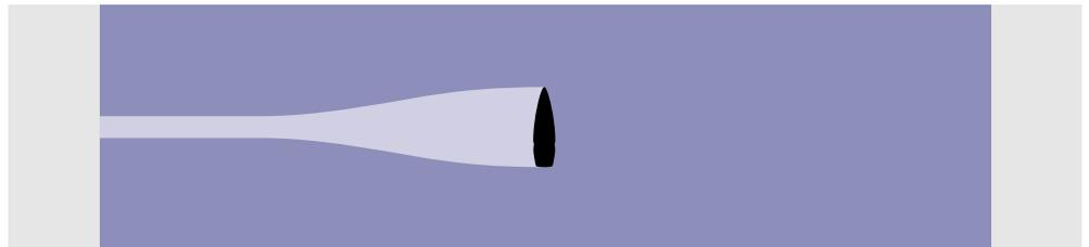
4. Bullet continues to penetrate target as it turns to produce increased 'cavitation' effect.
