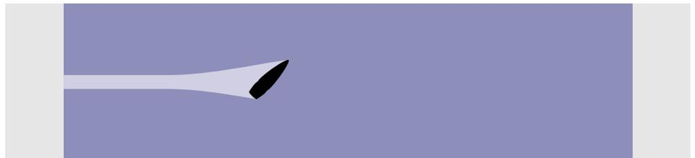
3. With weight of bullet concentrated at the base, it rotates so that heavier end faces forward.
